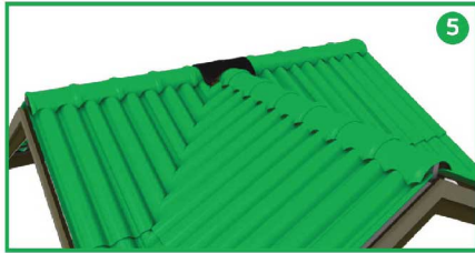
Put a piece of Trilon Dry Tech on the intersection to prevent water leakage.
